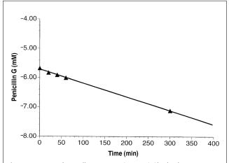
**Figure 4.** Kinetics of penicillin G in wine (pH 3.28), (the k value was 0.0047 min<sup>-1</sup> for five independent experiments, which included those in aqueous sulfuric acid and in red and white wines).
