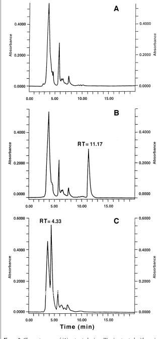
**Figure 2.** Chromatograms of (A) untreated wine, (B) wine treated with penicillin (3.4mM) at t = 0 min, and (C) a treated wine sample at t = 1185 min.
